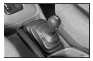
The transfer case shift lever is on the floor to the right of the driver. Use this lever to shift into and out of four-wheel drive. An indicator light comes on when the transfer case is in four-wheel drive. Your vehicle's transfer case shift lever may shake or vibrate. This is normal and your vehicle does not require service.
